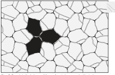
Step 3: Complete the balance of the surface to be covered with single pavers.
