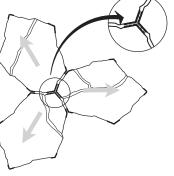
To make the installation easier, the front of the paver should point to the back of the other paver.
